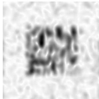
Fig. 5.9. A Wavelet Tour of Signal Processing, 3 rd ed. Directional Gabor wavelet transform |Wf(u, 2^j, \alpha)|^2 of a texture patch, at the scales 2^j = 2^{-4}, 2^{-5} , along two directions \alpha = 0, \pi/2 . The darker a pixel, the larger the wavelet coefficient amplitude.
