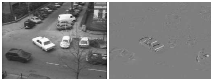
Fig. 12.16. A Wavelet Tour of Signal Processing, 3 rd ed. (a): Image of video sequences with three cars moving in a street. (b): Motion compensation error.
